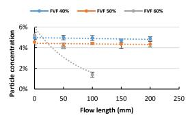
Figure 3: Particle concentration along flow length by different FVF
